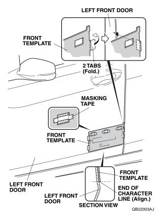
3. Align the front template with the end of the character line, and attach it to the left front door with strips of masking tape.
